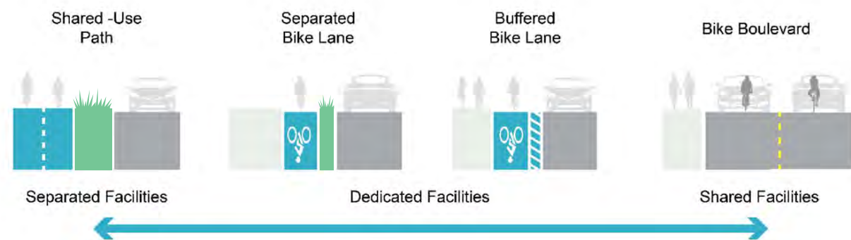
Figure 39 Bike Facility Degree of Separation
