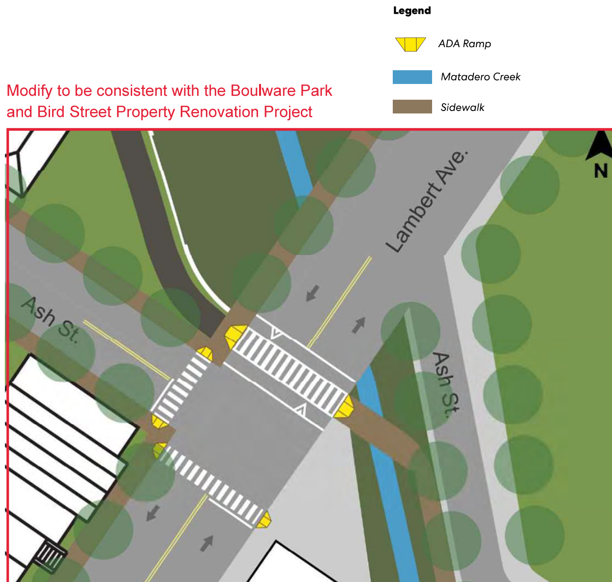
Figure 58 Lambert Avenue and Ash Street Conceptual Intersection Design
