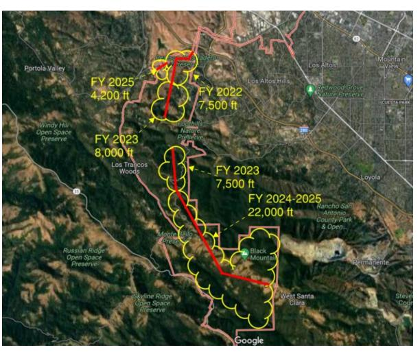
Our key mitigation activity is undergrounding eleven miles of electric lines in the Foothills area. This project involves installing substructure work, including boxes for electric and fiber lines; removing electric lines and fiber lines from poles; and installing padmount equipment where possible.
